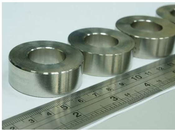
Fig. 7. Standard ring samples for RCT (a); microscopic captures (USB-microscope, max. magnification up to \times 300 ): one of the side surfaces of the ring specimen (b) and its representation in laser reflected beam (c)
