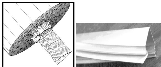
Figure 8. Twisting of the profile during extrusion: a – simulation results; b – photo of actual profile.
