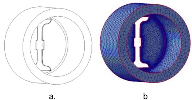
Figure 2. Flat die and container: a – solid model in CAD system; b – FE model ready for simulation
