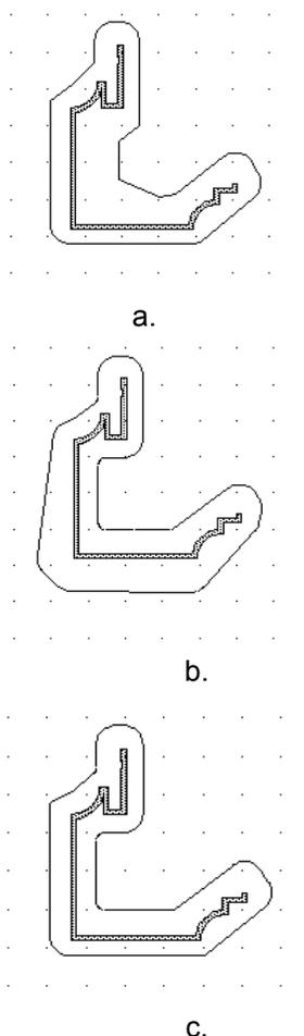
Figure 7 Three different variants of the feeder plate shape. Calculated profile twisting: a – 7.6 radian/m, b – 5.75 radian/m and c – 4.9 radian/m.
