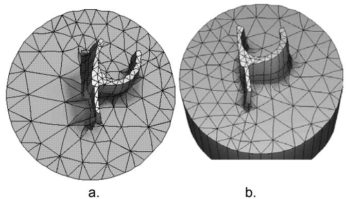
Figure 4 The influence of the orifice position on product bend simulated by 3D-model: product shape before (a) and after (b) optimisation of orifice position (deformation of the product is magnified).
