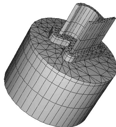
Figure 5. Shape of the product obtained after use of a chamber on the die (minimal bend and twist).
