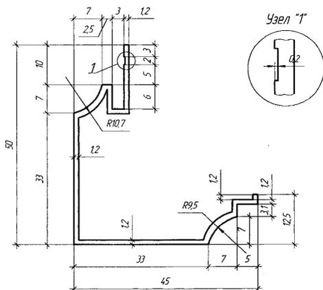
Figure 6 Drawing of the profile for building industry
