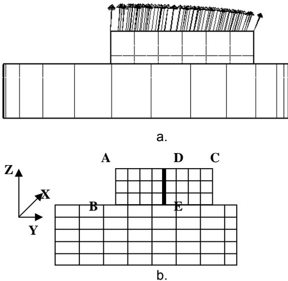
Figure 3. Velocity vectors at the end of the extruded product calculated by 3D-model (a) and the scheme of the algorithm for profile shape distortion evaluation (b).
