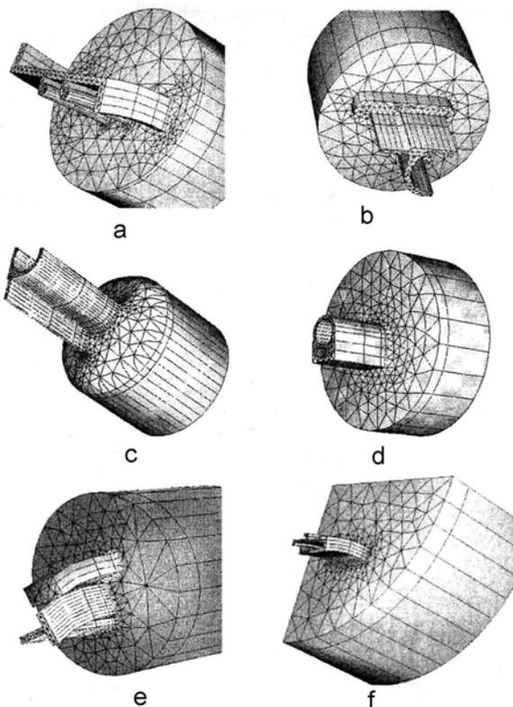
Figure 1. Different cases of profile extrusion: a – shear die; b – shear die with feeder plate; c – streamlined die; d – die with mandrell; e – multi holes die; multi-holes die with planes of symmetry
