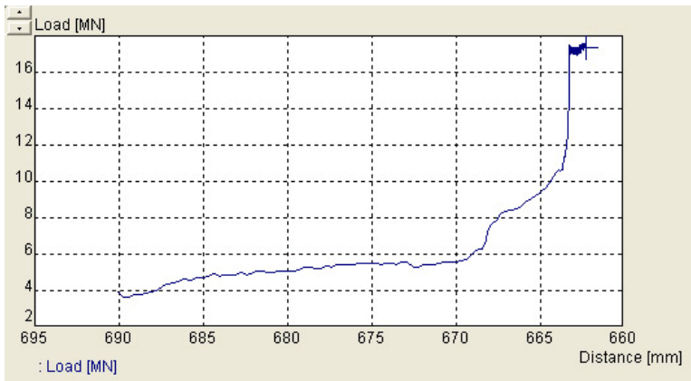
Figure 6: The graph of the load versus punch travel.
