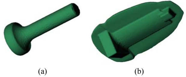
Figure 3. The billet after the first (a) and second (b) forging blows.
