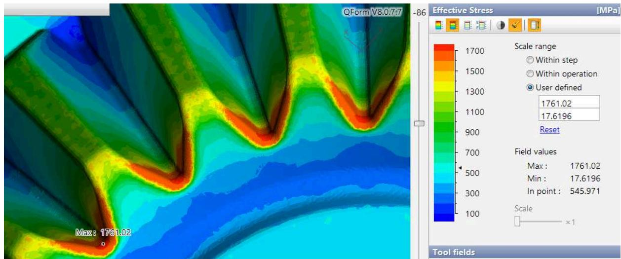
Fig. 3. Distribution of equivalent von Mises stresses (in MPa) in the upper die at the end of forging
