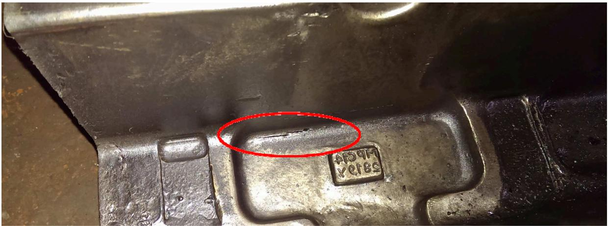
Fig. 6. The crack after about 200 forged parts in the third cavity of the die block in hot hammer forging.
