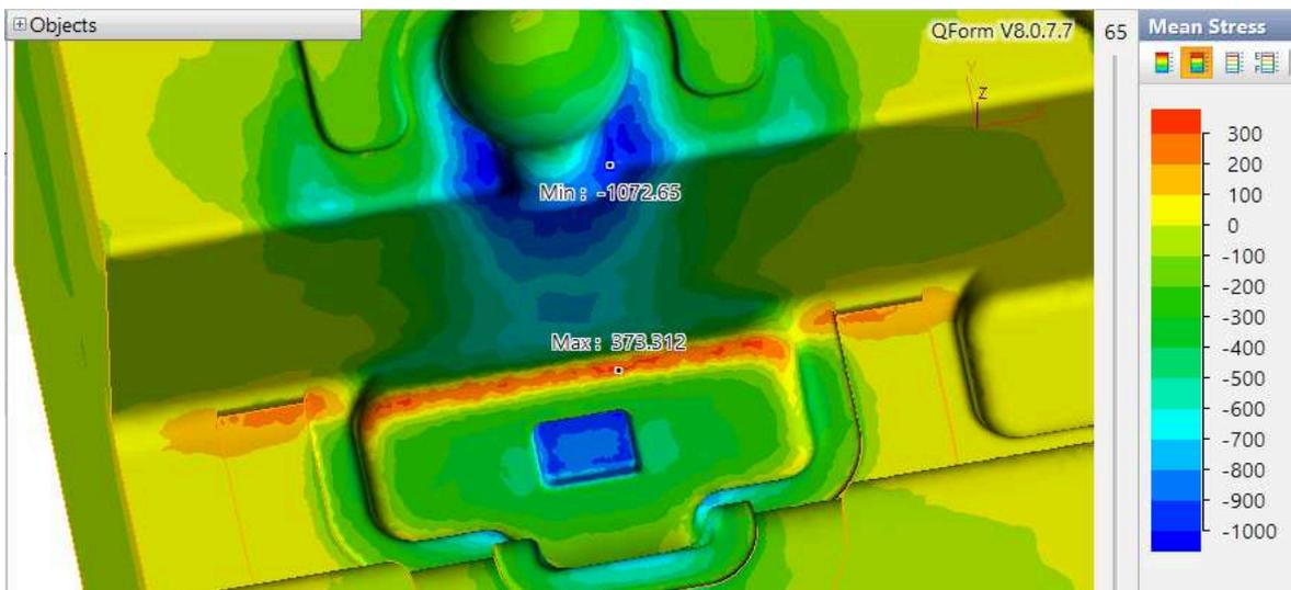
Fig. 7. The mean stress distribution and its extreme values are in the critical zone of the die during the third forging action.
