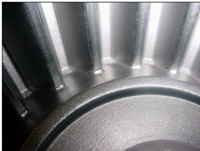
Fig. 2. The crack in the die appeared after 400-420 cycles
