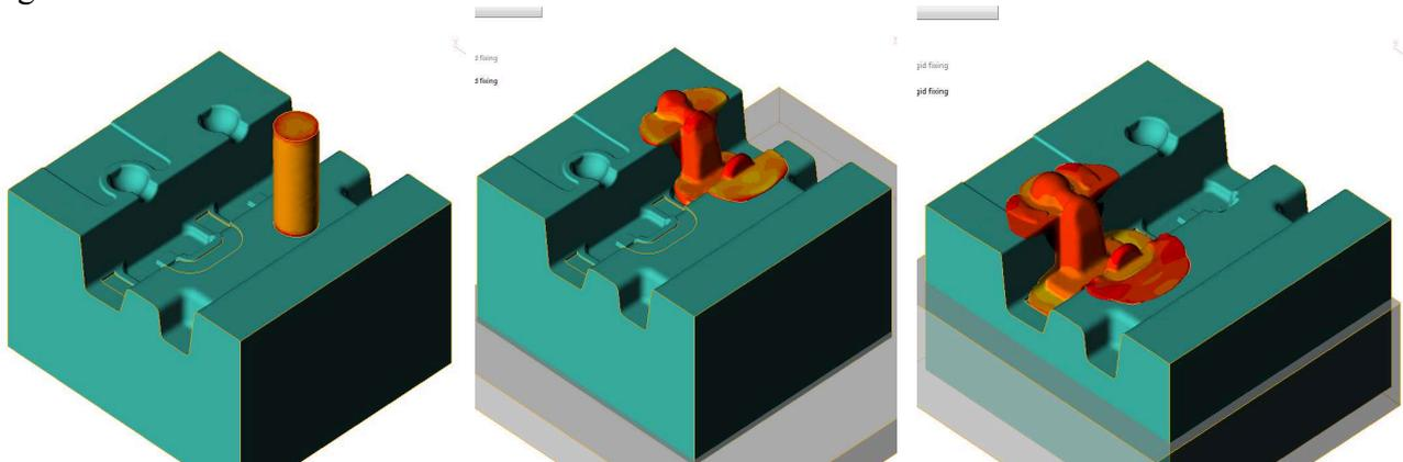
Fig. 5. The billet in the first, second and third blows of hot steel forging sequence.
