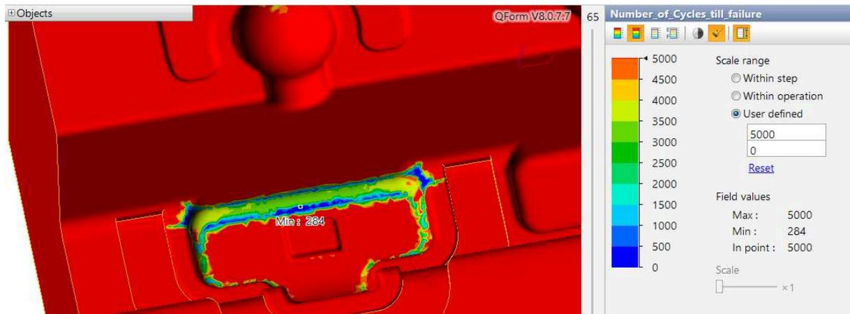
Fig. 8. Number of the cycles till the die failure because of LCF: minimum amount 284.
