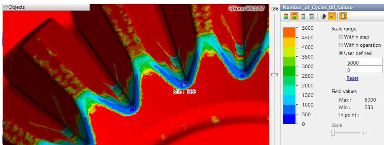
Fig. 4. Location of the crack predicted using proposed model with indication of the number of cycles till failure as 398.
