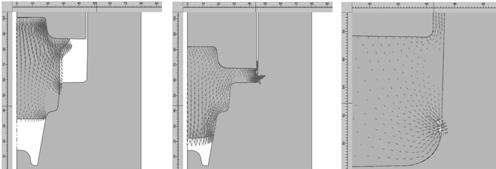
**Fig. 5:** Velocity distributions in isothermal near-net shape forging: a – initial position; b – intermediate stage with lap; c – lap (magnified view)
