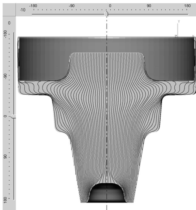
**Fig. 13:** Forging part macrostructure: a – experiment; b – FEM.
