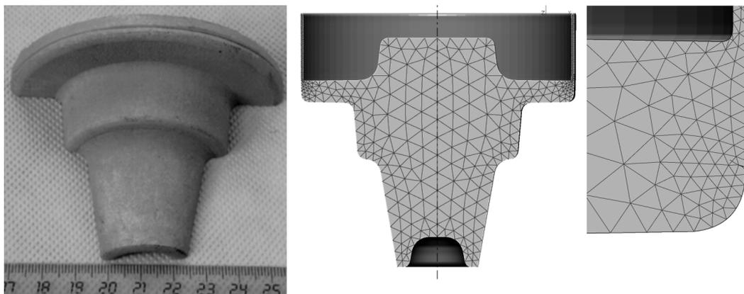
**Fig. 12:** Lap identification: a – experiment; b – FEM; c – lap (magnified view).
