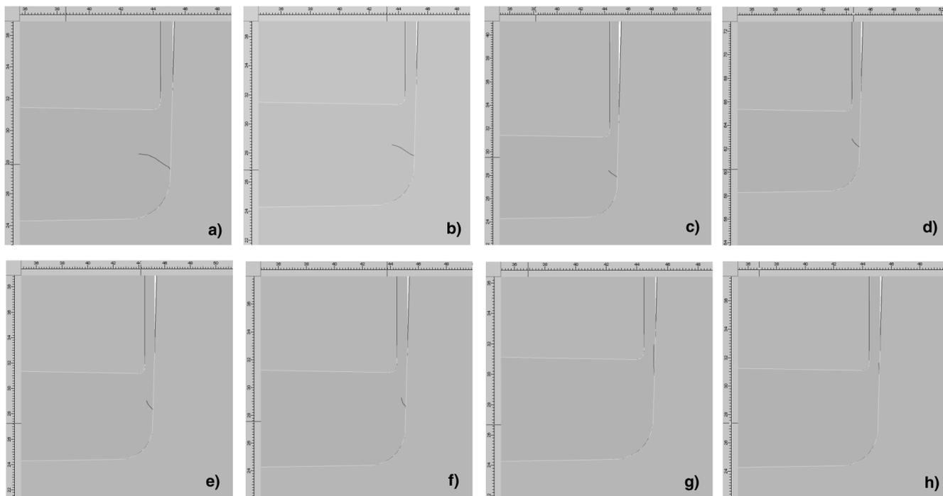
**Effect of temperature.** The results of the temperature effect on the simulation are shown in Fig. 9. It is seen that the temperature of the workpiece and correspondingly the dies temperature influence the forming load. The die velocity was constant and equal to 2 mm/s in all trials. Generally the forming load depends on part geometry, fric-
