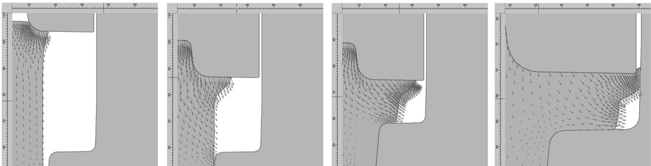
**Fig. 6:** Lap formation in forging process: a, b, c, d – stages of lap formation;
