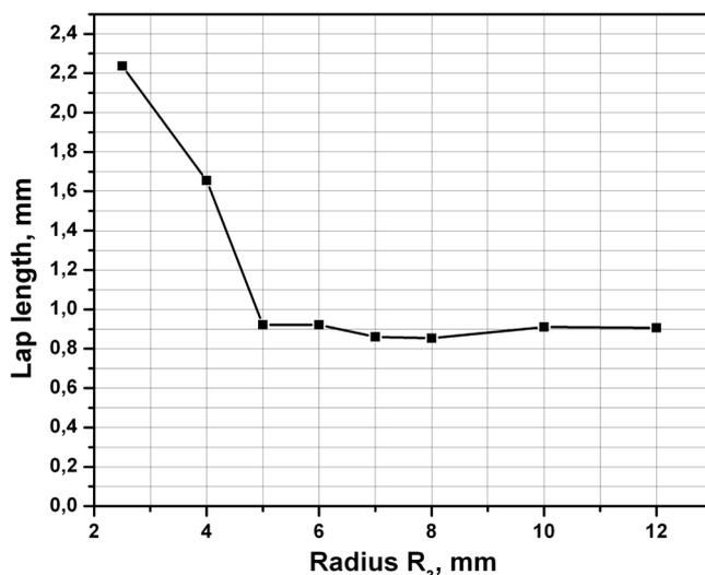
**Fig. 2:** Plot of the lap length versus radius
