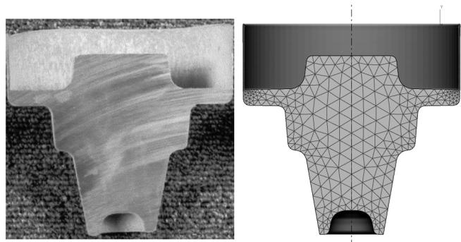
**Fig. 11:** Forging part with flange: a – experiment; b – FEM.
