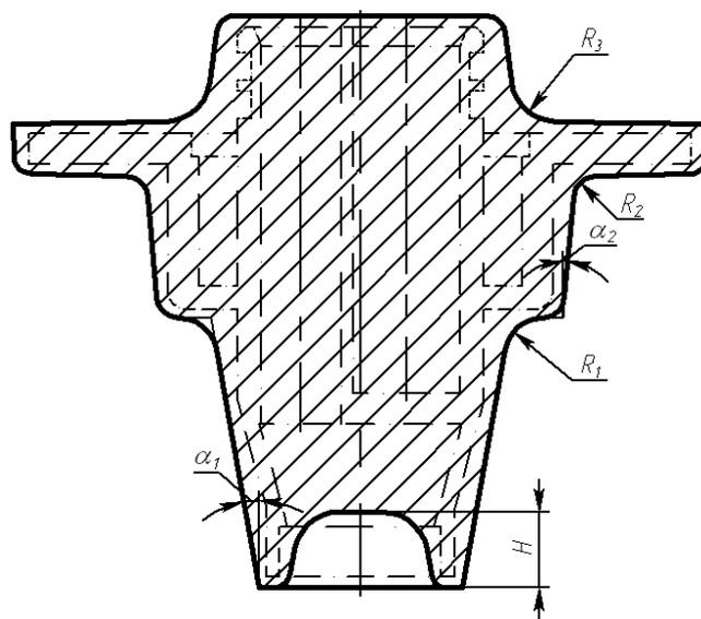
Fig. 1: Drawing of forged part (chain line corresponds to machined part)
