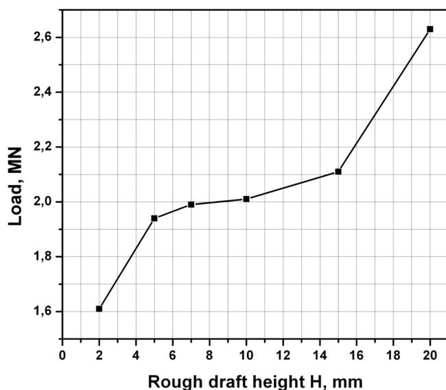
**Fig. 8:** Load versus rough draft height
