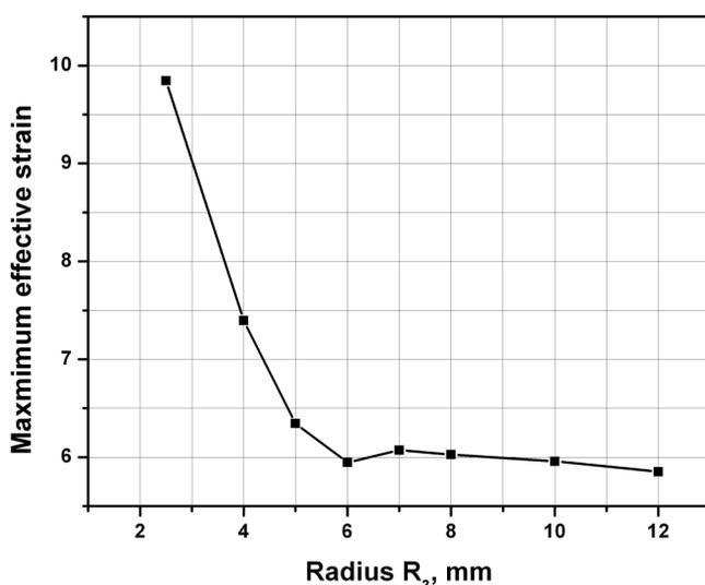
**Fig. 3:** Plot of the maximum effective strain versus radius
