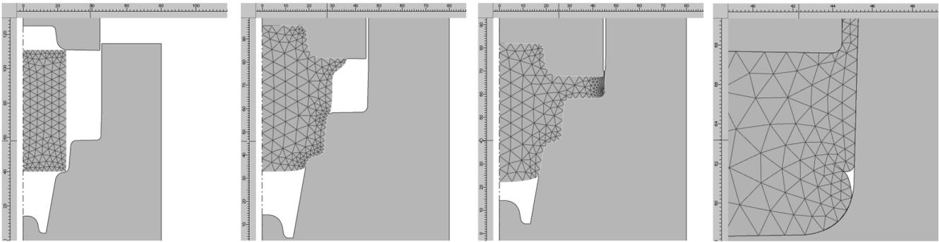
**Fig. 4:** Stages of metal forming process: a – initial position; b – intermediate stage; c – intermediate stage with lap; d – lap (magnified view)
