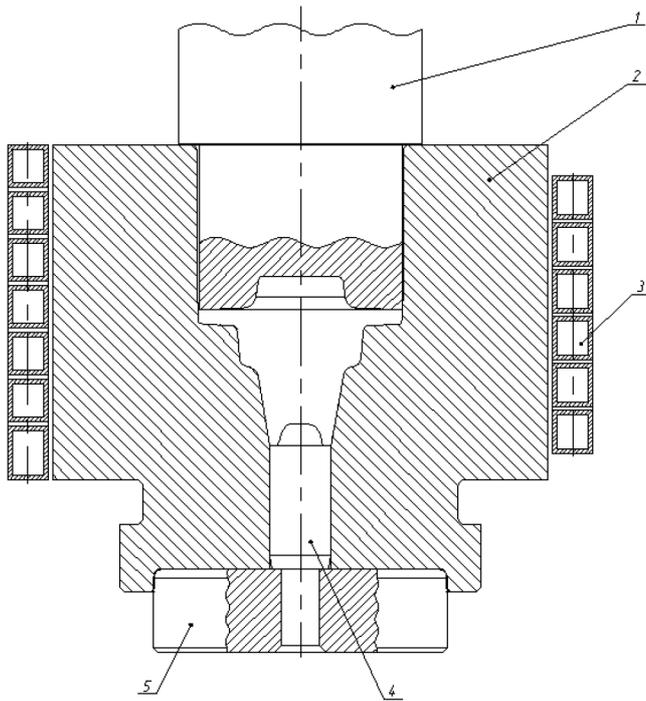
**Fig. 10:** Schematic view of isothermal enclosed die forging dies.
