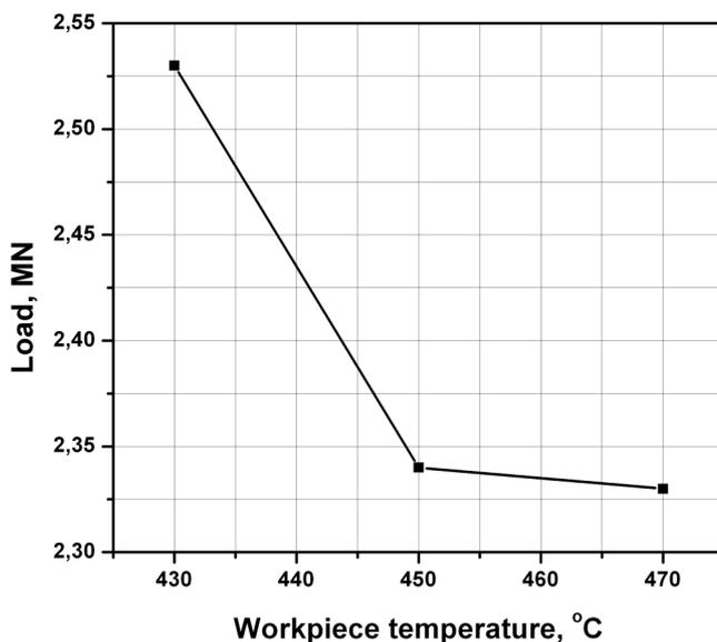
**Fig. 9:** Load versus workpiece temperature
