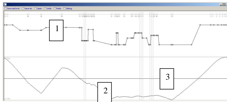
Figure 7: The evolutes of the bearing length (1), the profile velocity distribution (2) and average profile velocity shown as a line (3)
