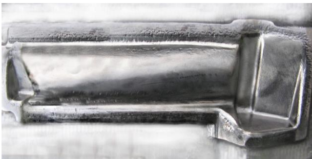
Figure 7. The lower finish die with the trace of intensive abrasive wear after forging of 300 parts.
