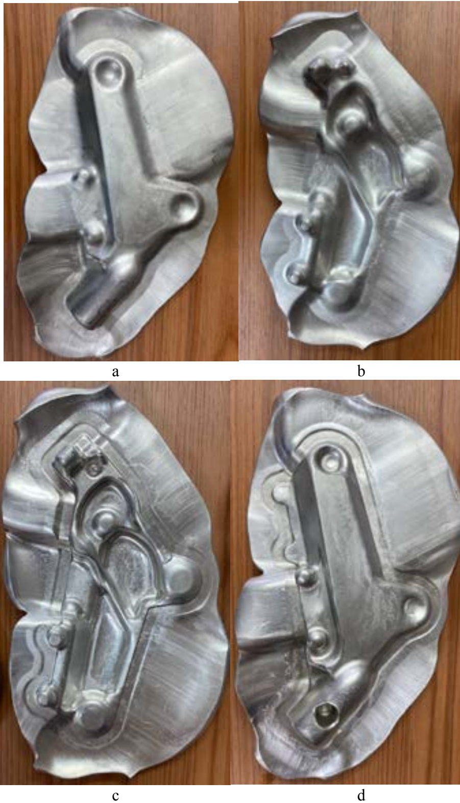
Fig. 7. Photo of the actual preform part top and bottom views (a, b) and finished part top and bottom views (c, d) forged using proposed technology (no material flow defects).
