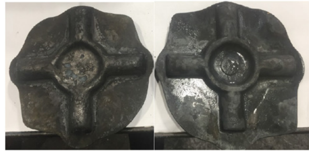
Fig. 4. Photo of the actual preform (a) and finished (b) forged parts using proposed preform shape (no material flow defects).
