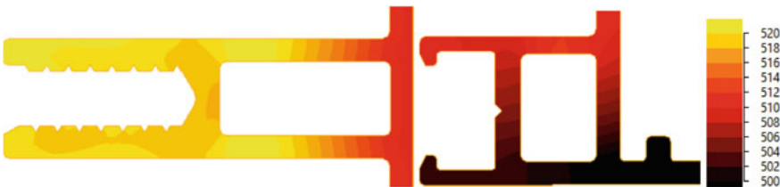
Fig. 6 The temperature distribution in samples #1 and #2. (Color figure online)
