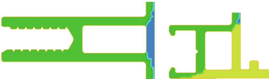
Fig. 5 Material streams in samples #1 and #2. The material from different streams is shown by different colors. (Color figure online)
