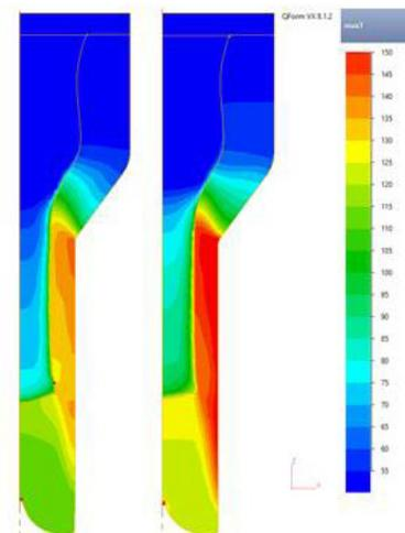
Fig. 8: Maximum temperature distribution in compacted PE. Extrusion of aluminum cup with inner diameter  $d=20$  mm and punch velocities  $v=50$  mm/s (left) and  $v=150$  mm/s (right) All simulation results are shown in table 1.
