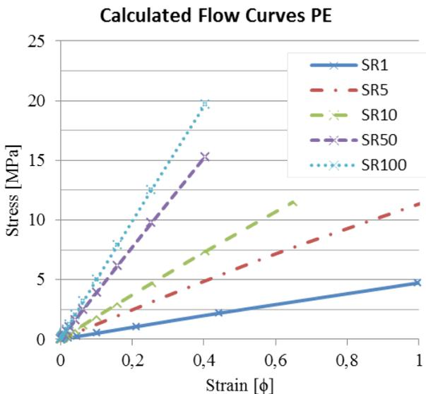
Fig. 4: Stress versus displacement for low density poly-ethylene ( $T = 190\text{ }^{\circ}\text{C}$ ), measured for different strain rates 1-100 s<sup>-1</sup>
