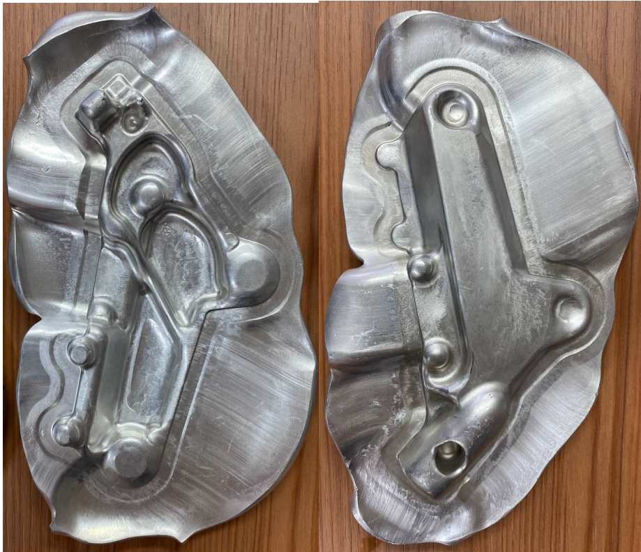
Fig. 7. Photo of the actual preform part top and bottom views (a, b) and finished part top and bottom views (c, d) forged using proposed technology (no material flow defects).
