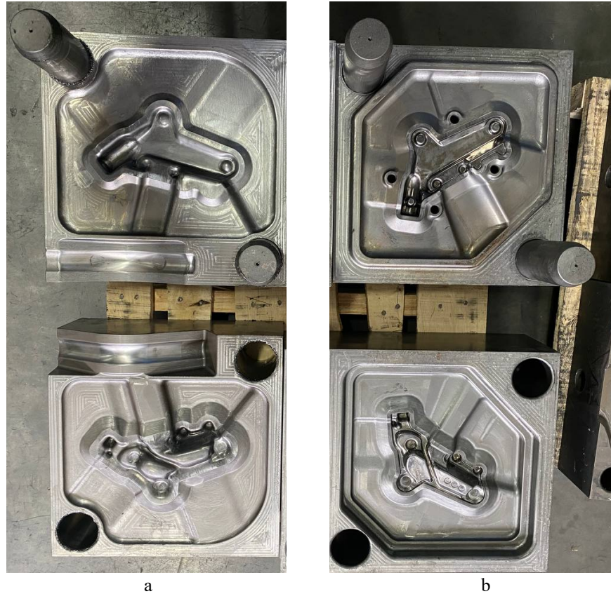
Fig. 6. Photo of the actual upper and bottom forming dies made using the QForm Direct die geometry export: preforming (a), finishing (b).
