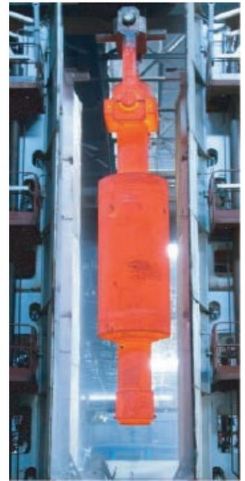
Quenching of the rotor in the sprayer device
