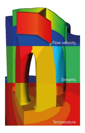
QForm Extrusion calculates material flow fully coupled with temperature and deformation of tool considering distortion of die set elements
